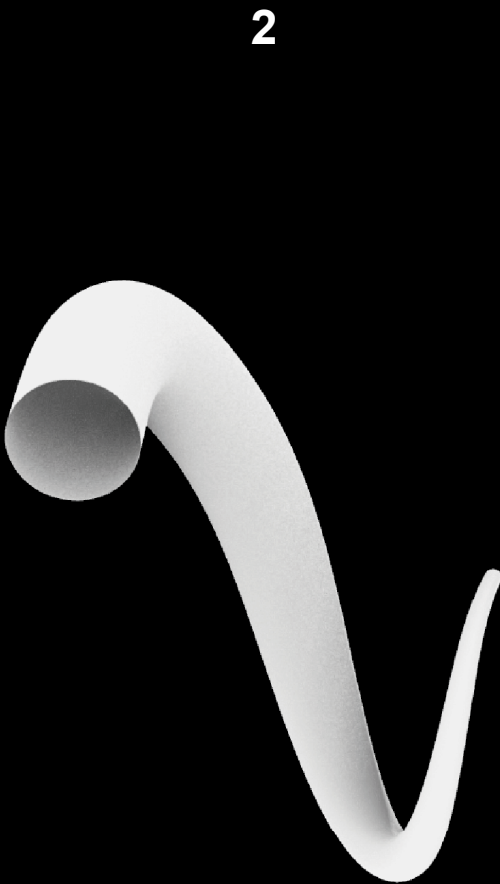
Piping applied to curve
